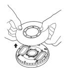
► Loosen the screws of the middle housing plate with an appropriate screwdriver and remove the plate .
